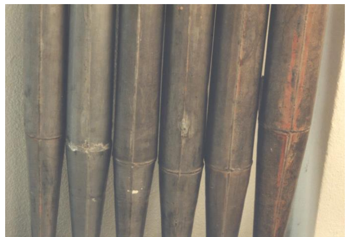
Rear view of the same pipes. The Lorentz former A pipe still displays the pipemakers red size along the soldered seams which was never washed of (frequently also seen in such pipes made by Herman & Eijzenmenger).
