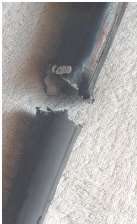
size (glue & white chalk) not being washed off the inside after soldering but accumulating moisture on the thin lead material
