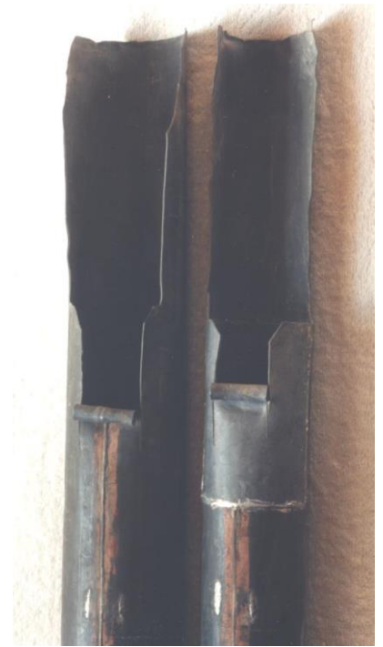
Lorentz led pipes E and C pitch radically altered by Frobenius by cutting tuning coils (E with new piece of rolled lead inserted)
