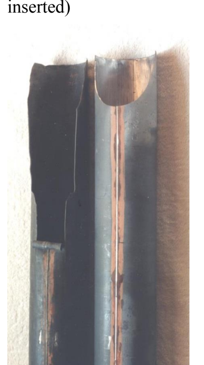
Left: C-pipe drastically retuned by coiling down - Right: my exact replica of this same pipe cut to correct C-pitch
