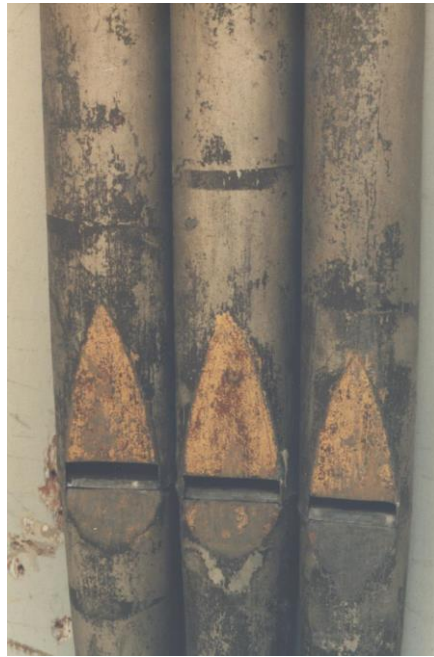
The Lorentz former Rückpositiv front pipes display astonishing well preserved mouths: low cut-up, no nicking
