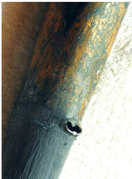
Damages on those 2 pipes as found in March 2000, just where new pipe foot tips were soldered on c. 1960. the new lower part disguised by paint. This calamity only stems from the pipemakers
