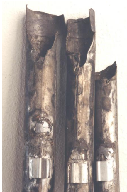
Brebosch normal front pipes, body lengths added to and hooks displaced for later re-arrangement
