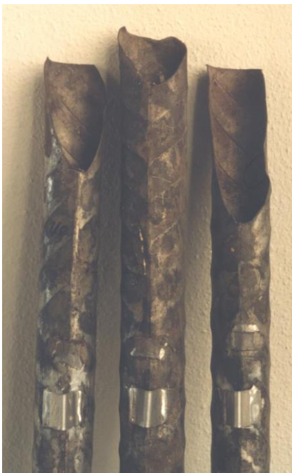
Brebosch dummy, embossed front pipes (the cutting out of rear top gives an illusion of speaking pipes, frequently encountered in antique organs)
